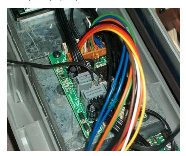
8. Attach 55027 decoder to double-stick tape. Connect plug to loco's main board. **Attention:** Do not reverse plug! Plug should clear three-pin connector on board.
