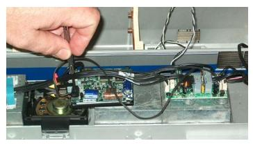
6. Plug the sound module power leads onto pins on loco's main board, then connect the stripped leads to screw posts on sound module (see Step 8 photo).
