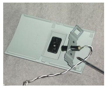
1. Remove the body shell and roof panel. Install the 65853 smoke unit in the roof panel. Plug the wire terminals onto pins labeled "Smoke" on loco's main board.
