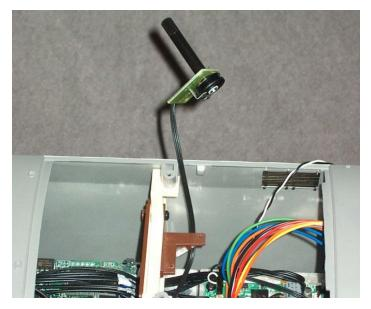
9. Plug the volume control cable into socket on sound module. Reinstall body shell.
