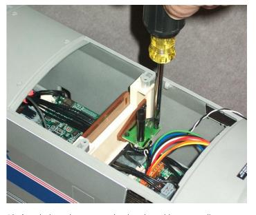
10. Attach the volume control to bracket with two small screws (from 69002). Reinstall roof panel.
