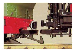
LGB "hook and loop" couplers are engineered for easy, reliable operation, even on uneven track sections.
