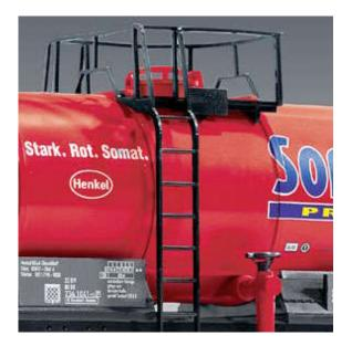
Ladders and other details on LGB trains are made of flexible materials to resist damage in accidents.
