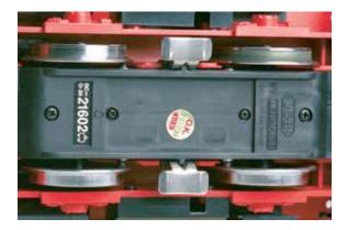
Critical, but hidden, LGB parts, like this gearbox, are made with glass-fiber reinforced composites.
