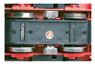
Critical LGB parts, like this gearbox, are made with glass-fiber reinforced composites.
