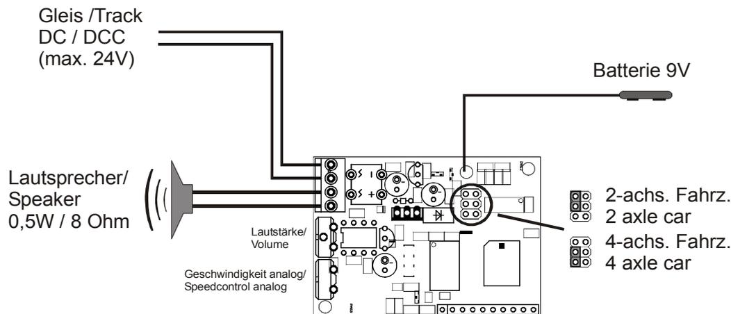
In digital operation, there is no need for the 9-volt battery. In analogue operation, a battery is required to ensure a pure sound even when travelling at slow speed. The volume and the speed (only in analogue operation) can be set via the two potentiometers next to the terminal screw bar. The coding bridge (see drawing) allows you to set whether you have a two-axle or a four-axle car. In digital operation, you can choose between 9999 addresses and 12, 28, or 128 rates of speed.
